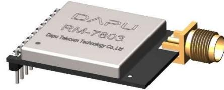
RM7803 Module is a Low power long distance transmission module, Adopted Semtec's High performance spread spectrum RF chip SX1278, for ultra long distance spread spectrum communication, Strong anti-interference and high receiving sensitivity over - 142dBm. At the same time, STM32l0 low-power MCU is embedded in the module to minimize the current consumption.
