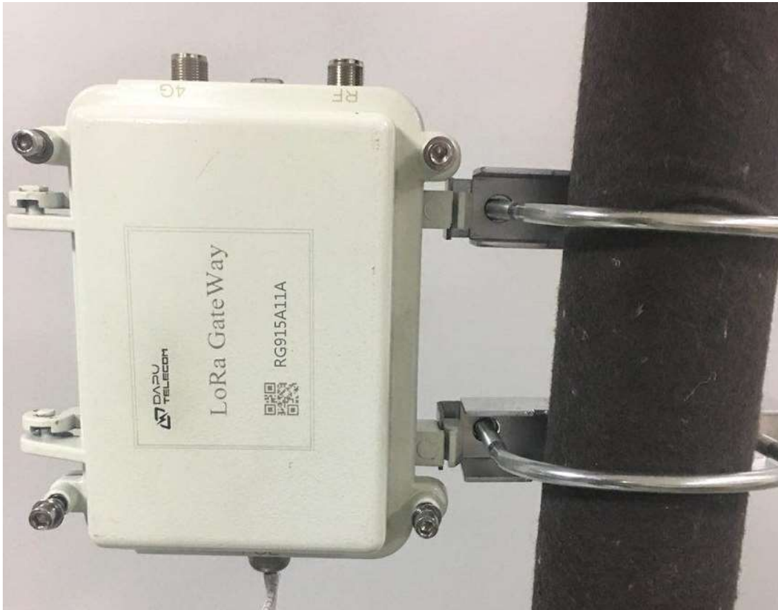
Figure 5-2: Gateway Installation diagram
